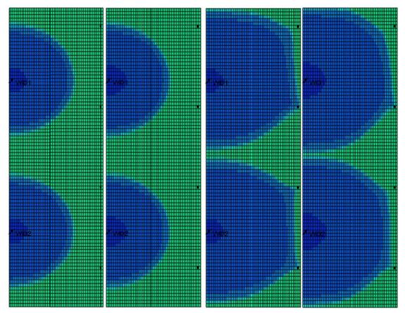
Figure 2. Water saturation fronts. 1) T=5 years, constant perm -2) Sw-dependent perm. 3) T=20 years, constant perm -4) Sw-dependent perm
