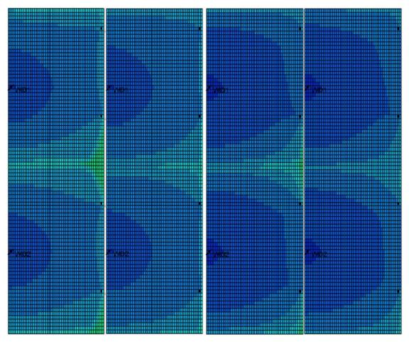
Figure 3. Water saturation fronts. 1) T=32 years, constant perm -2) Sw-dependent perm. 3) T=44 years, constant perm -4) Sw-dependent perm
