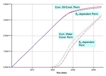
Figure 1. Cumulative production of oil and water. Comparison constant and Sw-dependent permeability
