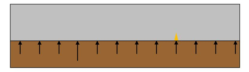
Compaction waves in overburden will follow "paths of weakness" to surface. These can develop as part of the process
