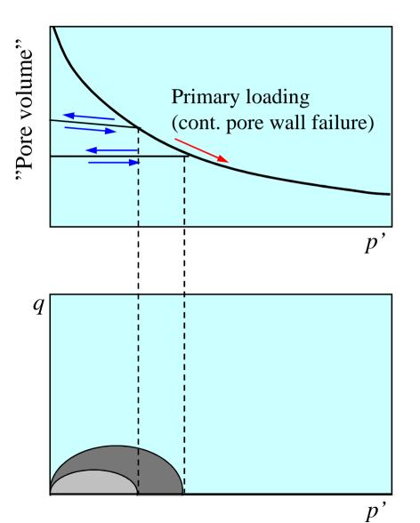
In stress-space (using *p* ' and *q*), we have a "safe" region, where material behaves elastic (grey). Unloading – reloading is within this region.
