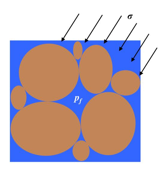
In a porous rock, the main mechanism is deformation of the pore space, not the solid itself.
