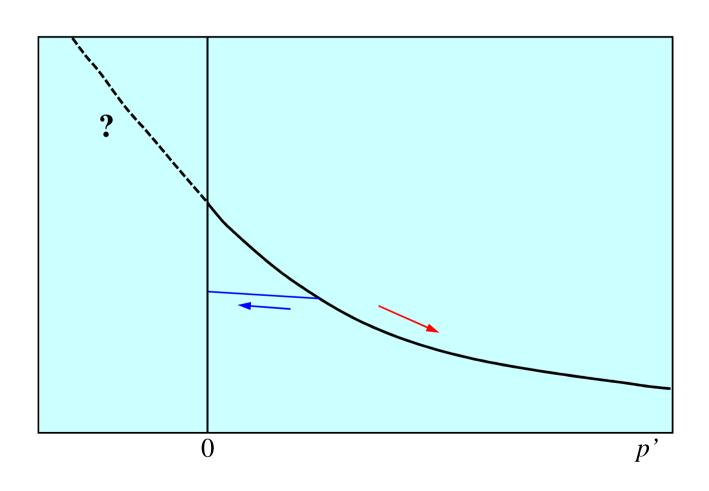
Definitely wrong. Primary loading curve is only valid for *increasing* mean effective stress
