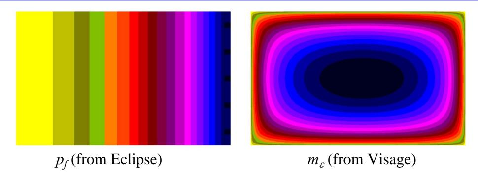
Although  $p_f(x)$  is very unsymmetric,  $m_{\varepsilon}$  is almost symmetric. This is an indication that BCs have a stronger influence than the process, and that  $\Delta f_D$  is indeed small.
