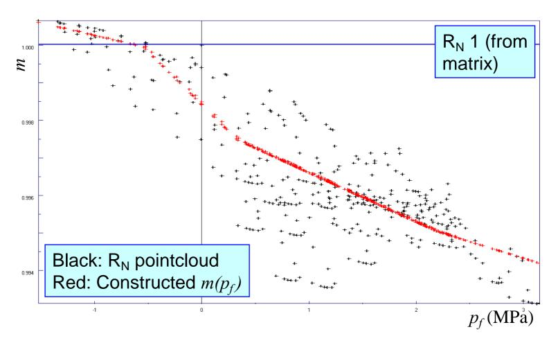
Material boundary  $R_N$ , typically larger spread, does *not* pass through (0,1)
