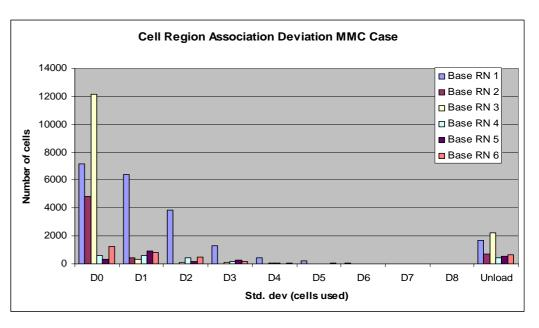
For each grid cell, the "standard deviation" of assigned ROCKNUM from different stress steps has been computed. The columns show #cells vs. stddev, SM left, MMC right (Unloading data are regarded as unsuitable for ROCKNUM assignment)
