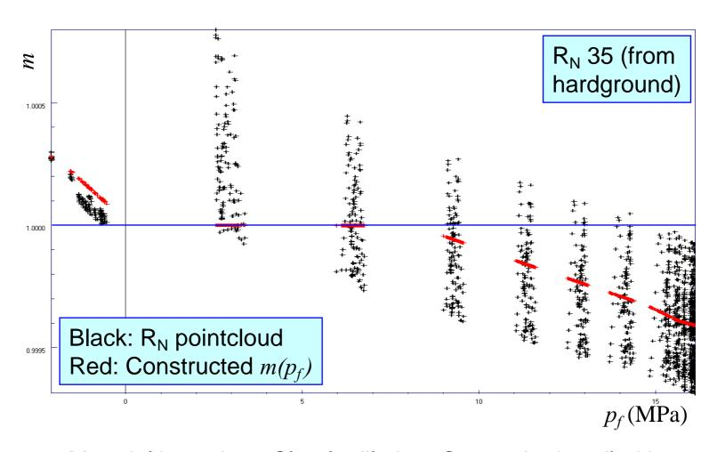
Material boundary. Clearly dilation. Cannot be handled by Eclipse, and must be disregarded
